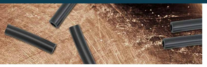
Halogen free, high density heat shrink tubing specially designed to meet the form stable demands in automotive battery cable and ground strap areas, highly abrasion resistant.
